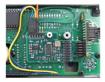
Four additional wire connections are needed by the MAB. Three of these wires are attached to the K2 front panel board, and the fourth wire is attached to the K2 control board.
