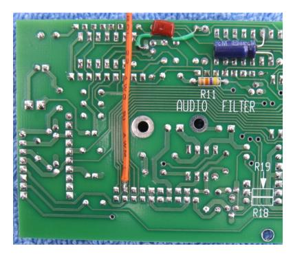
An orange wire is soldered to the K2 control board as shown.
