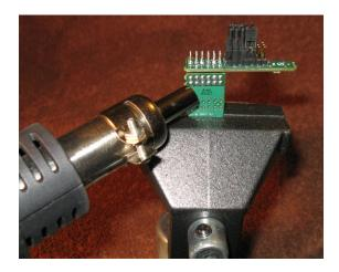
Once the solder melted it was easy to remove P1 with no damage while it was still soldered to the other board.
