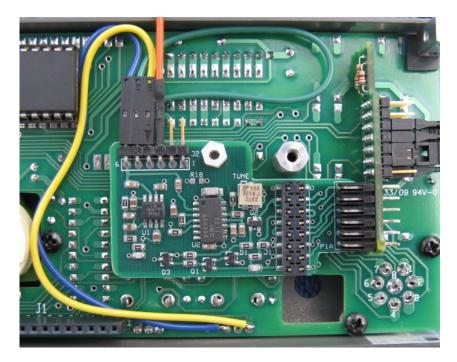
The K2 control board is then installed.
