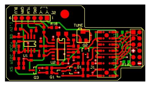
The layout is for a four-layer board with internal 5V power and ground planes. It was prepared using the free ExpressPCB<sup>9</sup> software.
