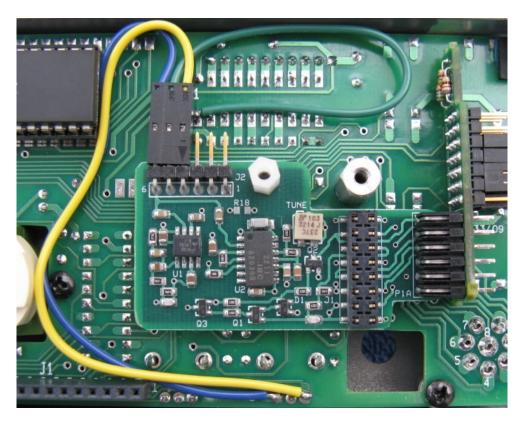
The three-wire front-panel-board cable assembly is prepared and installed as shown above. The wire colors were selected in accordance with the standard resistor color code and which J2 pin they are connected to, e.g. the yellow wire goes to pin 4, the green wire goes to pin 5, etc.
