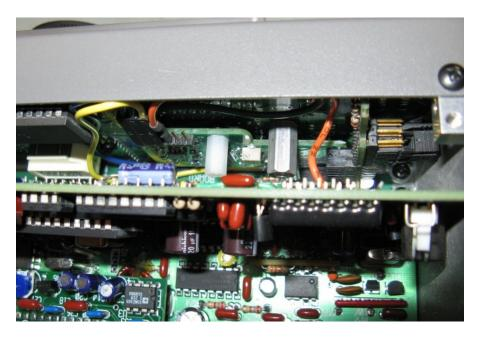
A nylon machine screw is used to secure the MAB to the K2 control board.
